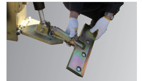
Quick and easy replacement of cutting head and blade.
